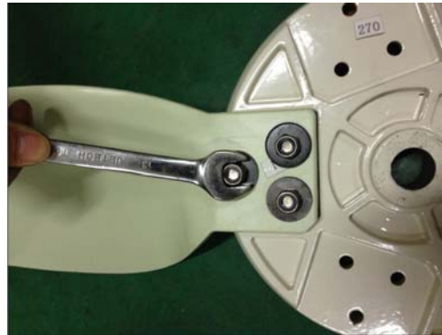
⑤ Place blade, flat washer and nylock nut, and tighten the nut to 18N.m
