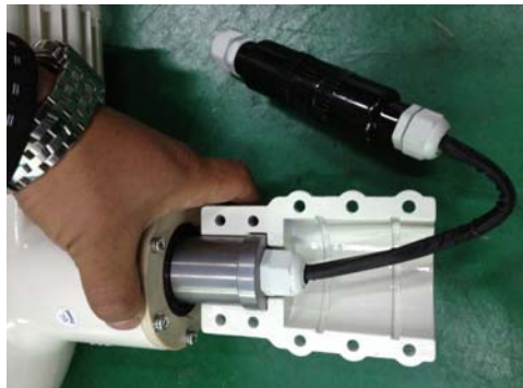
② Place rotating shaft on the upper part of the clamp.
