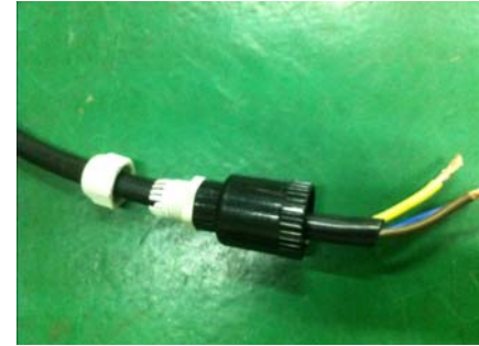
③ Pass the wires through the cover.
