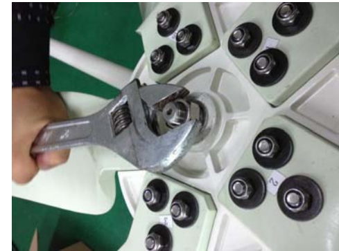
③ Fully tighten the nut to 154N.m
