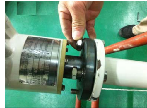
③ Place flat washer, spring washer and nut, tighten the nut to 37N.m
